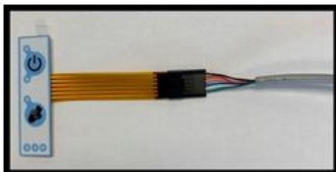
**Figure 1: Membrane Switch and Connector**
