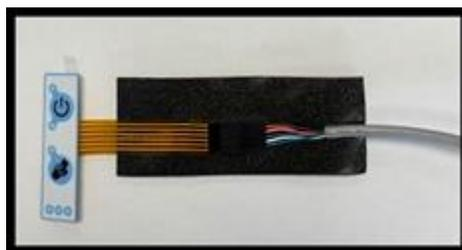
**Figure 2: Position Membrane Switch**
