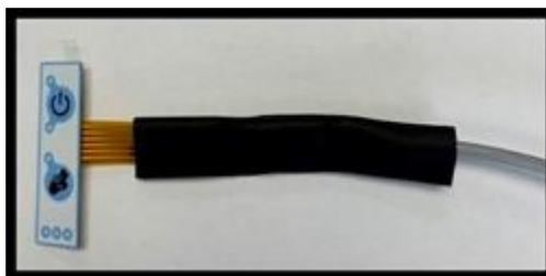
**Figure 3: Wrapped Membrane Switch with Pinched Ends, Eliminating All Gaps**
