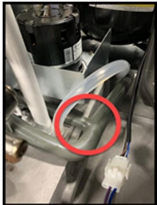
Figure 3: Intersection between drip tray and purge valve tubing
